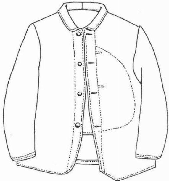
FIG 12. J. T. Martin 18 October 1864 contract lined sack coat (Cincinnati Depot). Perhaps the most common sack coat in modern collections, this coat exhibits features common to Martin coats: narrow ⅝" cuff stitching and shallow cuff slits (compare these to the Danish exchange coat), facing seam tapering to ¼", and sewn box stays on the pocket. This coat is of 3-piece construction and is heavily machine sewn. Lining is loose gray flannel and is hemmed on the bottom. Sleeves are marked with contract "J. T. MARTIN OCT-18-64" and inspector marks. "GEO.B.FRY, U.S. INSP. CINTI O." in separate sleeve linings. Note how the skirt corners do not match. (Smithsonian Institution)
