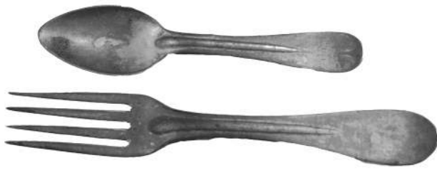
FIG 5. A fork (top) and a spoon (bottom) made completely of stamped sheet iron.
